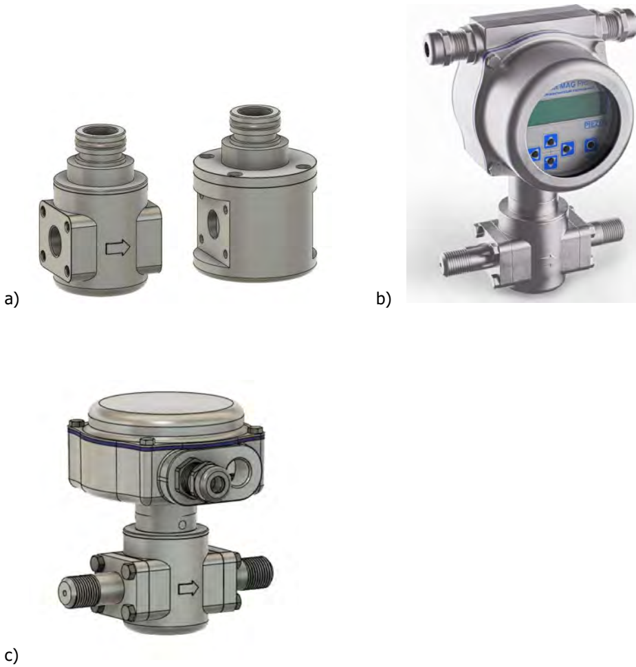
Figure B.12 Sensor design for small Dn diameters: a) remote design with connector; b) compact design with small-sized EM; c) remote compact design (with junction box)
