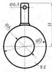
Figure B.10 Overall dimensions of grounding discs (rings) for flanged connections with Dn from 700 mm (A, D, H dimensions are for reference)
