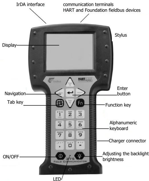
Figure E.1 - Model 375 communicator controls descriptions
