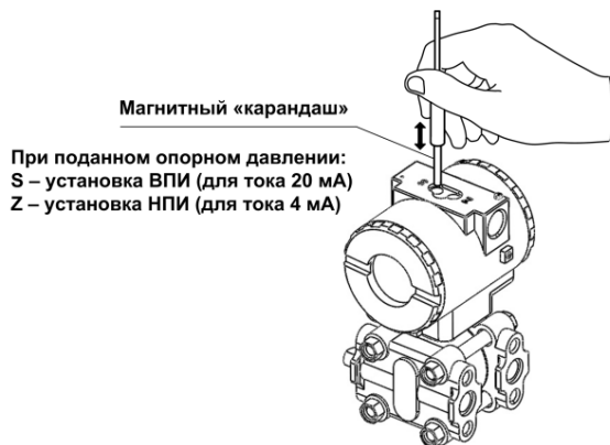
Figure 6.2. Location of Z (zero) and S (span) controls, local configuration
